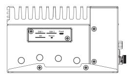
There are some ports SIM1, SIM2, Flash, M-SD Card and Recovery Button are placed on the side panel. It has a case cover these ports.
