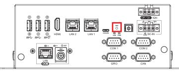
If the system have error or frozen status, you can press Reset Button to restart, then the system will reboot OS.
