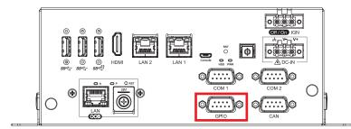
The power voltage of each GPIO pin is 0V to 3.3V. The maximum current can be 20uA.
