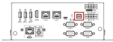
The Power Button is a non-latched switch with dual color LED indication.
