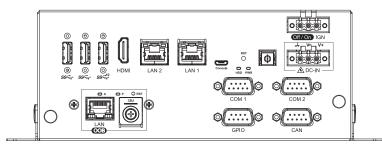
In Vecow EAC-6000-OOB series, Most of the I/O connectors are located on the front panels. Most of the general connections to computer devices, such as POWER CON, IGN CON, COM, USB 3.0, LAN (RJ-45), Digital Display Port, GPIO, POWER BUTTON, RESET BUTTON, LED indicators are placed on the front panel.
