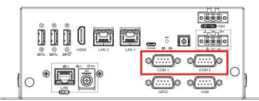
The COM 1,2 can be configured for RS-232, RS-422, or RS-485 with auto flow control communication. The default definition of COM 1 and COM2 is RS-232; if you want to use RS-422 or RS-485, you have to change COM mode the DIP Switch mode select.
