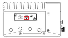
Press the Button enter Force Recovery Mode. Button is held down while either system is first powered on, or by pressing & releasing reset button while Recovery button is pressed.
