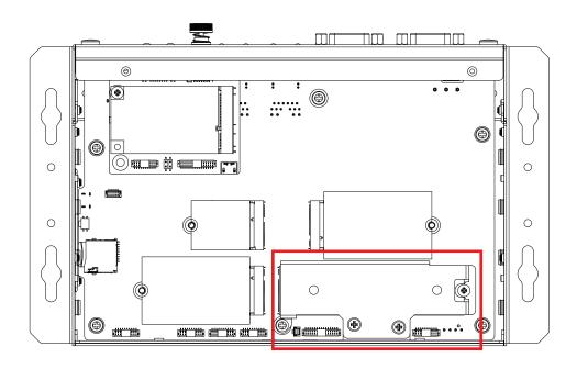
Step 3 Fasten one pan head M3x4L screw and two F-M3x4L screw.
