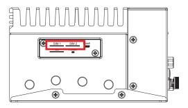
The external Nano SIM card offers wireless communication capability by M.2 key B 4G/5G Card to the system.
