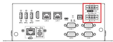
EAC-6000-OOB supports 9V to 50V DC wide range power input by terminal block. It can be divided into Top layer and Bottom layer. The Top layer is Ignition signal control application, and the bottom layer is power source input.
