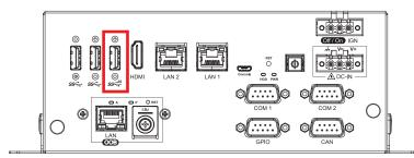
There is a USB 3.2 Connector connections available supporting up to 10Gb per second data rate in the front side of EAC-6000-OOB series. It also compliant with the requirements of Super Speed (SS), high speed (HS), full speed (FS) and low speed (LS).
