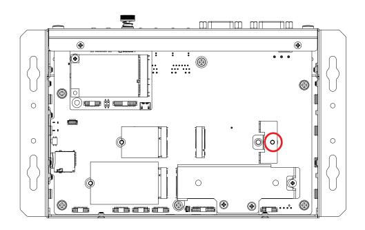
**Step 2** Install M.2 Key B 3042 into slot and fasten one pan head M3x4L screw.
