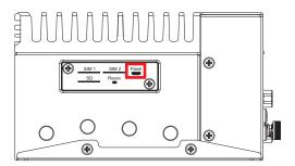
The EAC-6000-OOB USB Recovery mode provides an alternate boot device (USB). In this mode, the system is connected to a host system and boots over USB. This is used when a new image needs to be flashed. USB0 must be available to use as USB Device for USB Recovery Mode.
