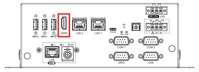
The Digital Display Port(HDMI) support HDMI V2.0 interface, connection supports up to Up to 3840 x 2160 @60Hz.
