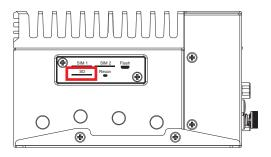
The external Micro SD card provides additional storage expansion. It is located behind the cover-plate on the front panel.
