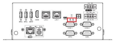
The HDD LED is presented with the storage active status. The PWR LED is presented with power of system is ready.on.normally.
