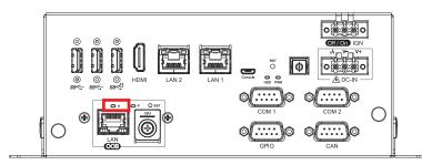
The LED indicator can instantly judge the power status of OOB Enabler and the connection status of OOB Enabler and Allxon Portal. If both LEDs are on, it means OOB Enabler is running and the connection to Allxon Cloud is stable.
