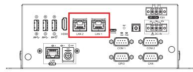
There are two 8-pin RJ-45 jacks supporting 10/100/1000 Mbps Ethernet connections on the front side of EAC-6000-OOB series. It supports 1000BASE-T gigabit data signals over standard Ethernet Cat 5/Cat 6 cable.
