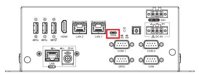
The Console Port is debug Port of system, it connected by Micro USB connector It can be connected by USB (Type A to Micro USB Type) Cable to USB Port of PC, and execute terminal tool, then it will get the system status message.
